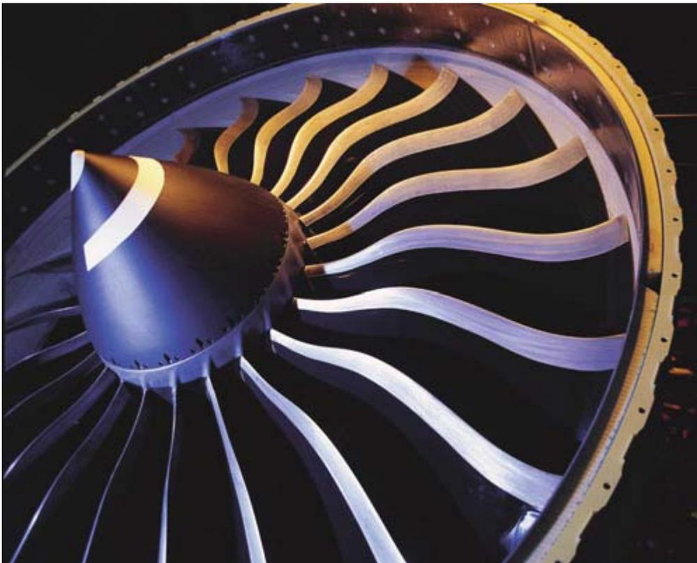
Blades of GENx engine are made of carbon fiber/epoxy composites (Krishan K. Chawla Composite Materials. Science and Engineering. New York: Springer, 2013. 552 p.)
