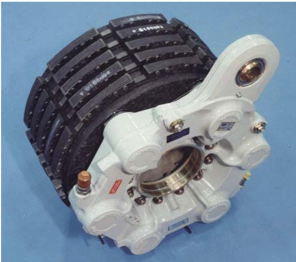
A carbon/carbon brake assembly that is used on a Boeing 767 airplane
