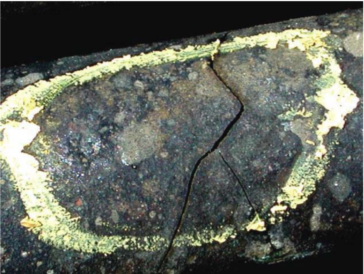
Cracks in Admiralty brass tube.
