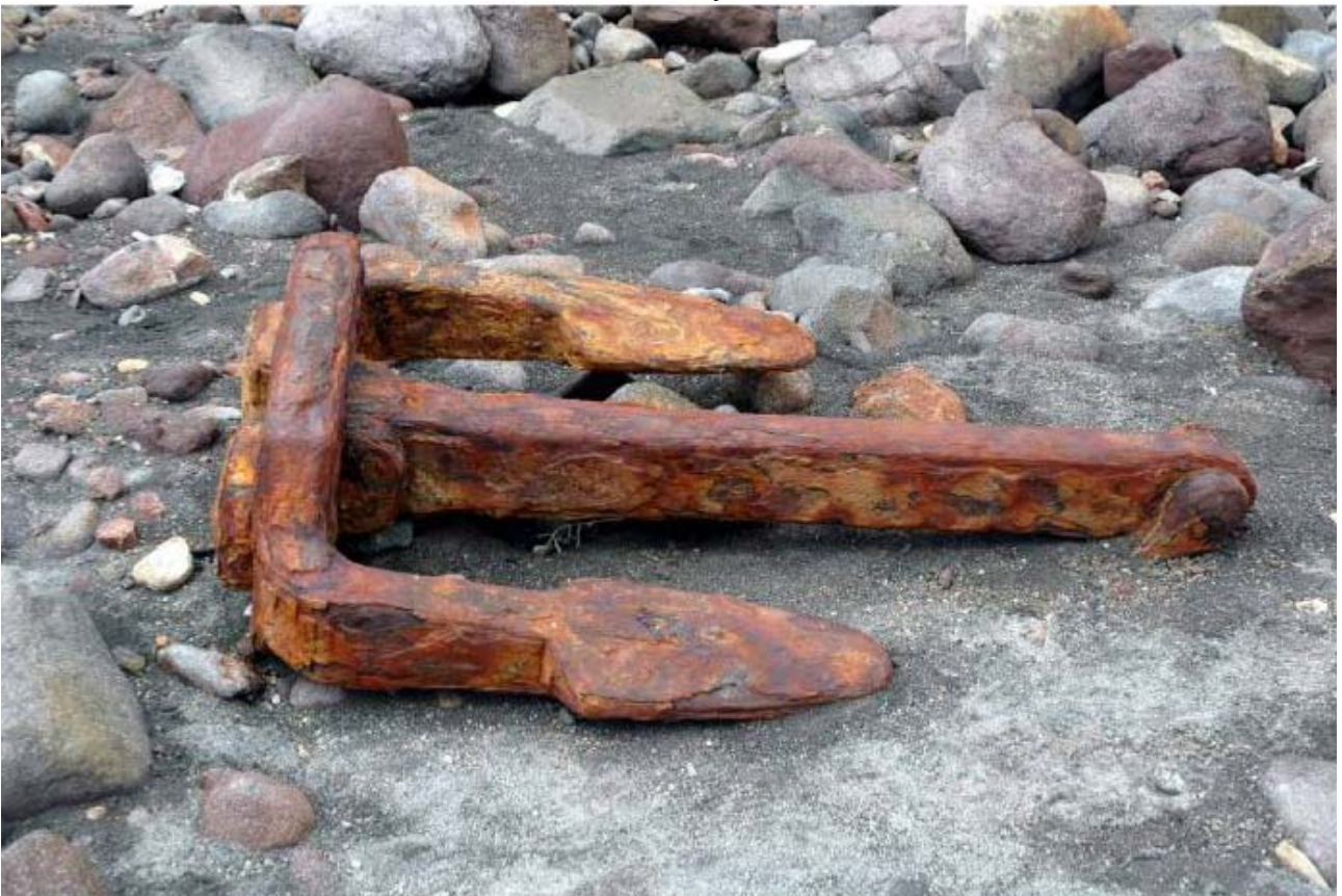
Corroded anchor made of carbon steel
