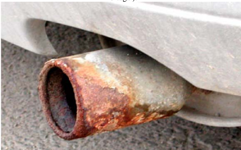
The exhaust system of a vehicle after dewpoint corrosion.
